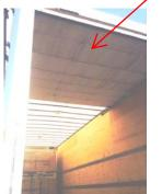
Wooden sides in linen delivery truck do not allow for effective cleaning
