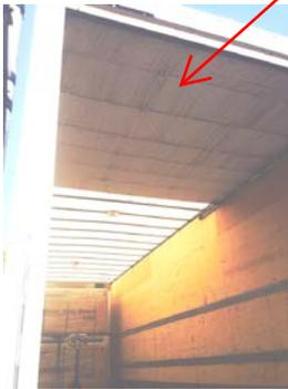
✘ Wooden sides in linen delivery truck do not allow for effective cleaning
